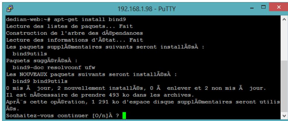
The screenshot shows a PuTTY terminal window titled "192.168.1.98 - PuTTY". The command "apt-get install bind9" is run, and the terminal displays the standard aptitude progress messages. It lists packages to be installed (bind9utils, bind9-doc, resolvconf, ufw), packages to be upgraded (bind9), and the total disk space required (493 ko). At the bottom, it asks "Souhaitez-vous continuer [O/n] ?" (Do you want to continue [Y/n]?).
